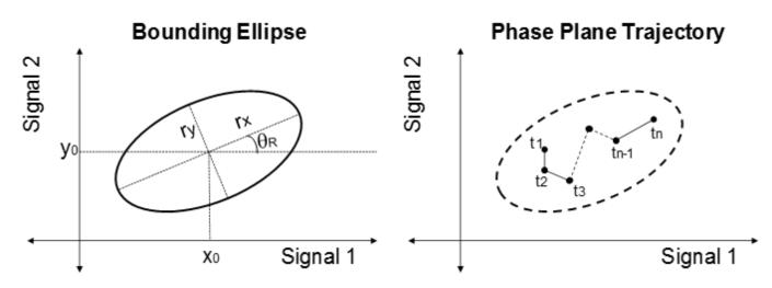
The X-Y plane is the phase plane defined by the two signals.  $r_x$  and  $r_y$  are the radii of the bounding ellipse along the x and y axes, and  $\theta_R$  is the rotation of the ellipse about the center. The ellipse center is at  $(x_0, y_0)$ . In the image, the phase plane trajectory of the signals lies within the bounding ellipse for all time-points  $t_1$  to  $t_n$ .
